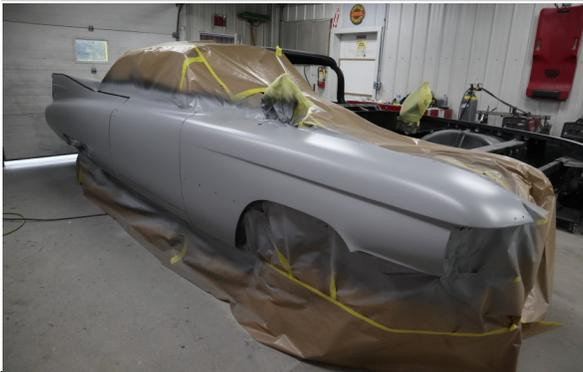
Jason and Jake have worked diligently to save the body of this old Cadillac. The exterior finish is really taking shape now as it's being worked through the multiple coats of primer and block sanding. Soon it will start getting edged with the original shade of Breton Blue that it came with from the factory. This one has been a long challenging process, but it's starting to look like a car again! Watch for the color photos and more updates soon on this restoration.
